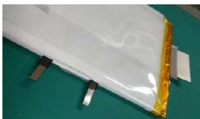
Specific cell integrating a heater for internal-short-circuit tests
