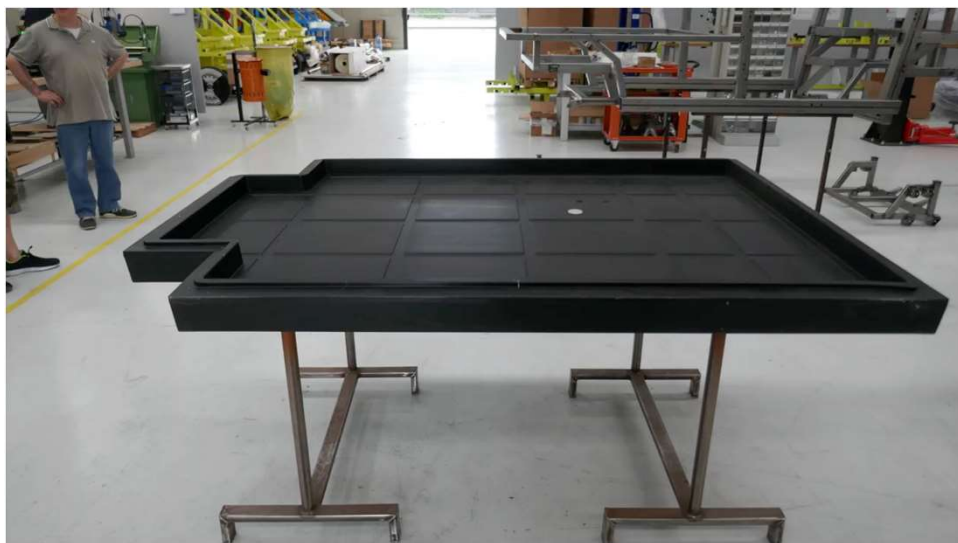
Ultra lightweight thermally insulated battery tray also acting as vehicle floor.
