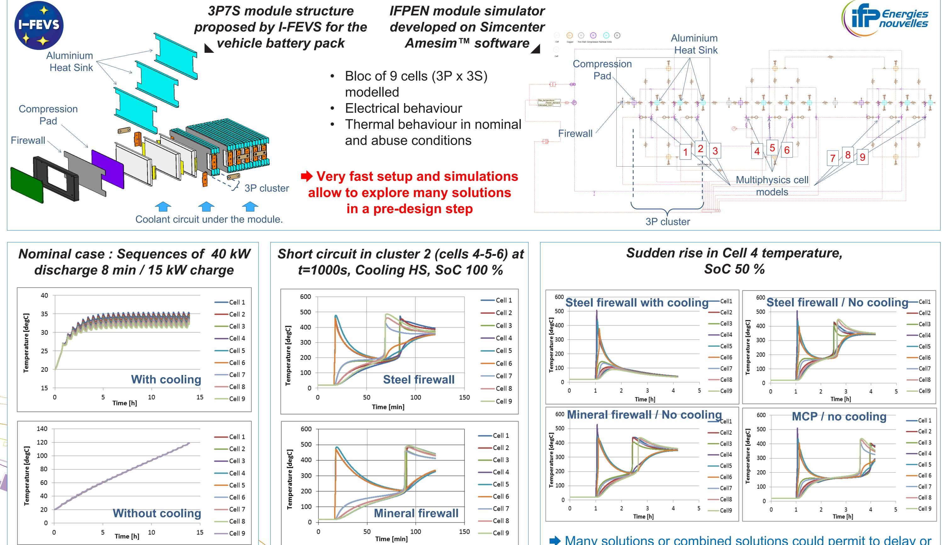
No thermal runaway after 15h of cycling in both cases Cooling allow to stabilize the temperature below 35 °C
